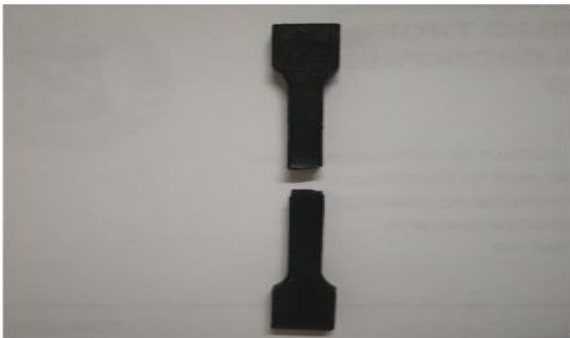
Fig 7 Tensile tested Sample
