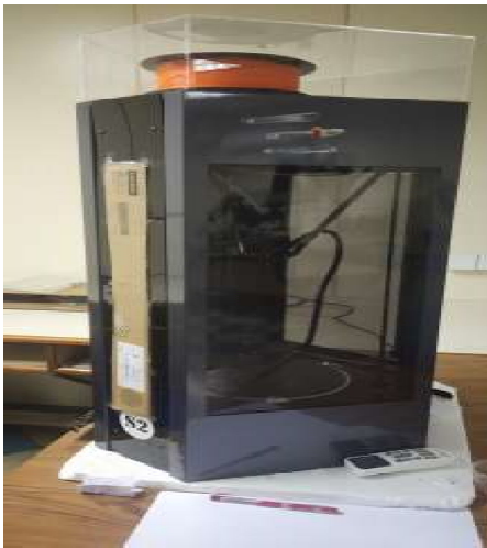
Fig 1 Fused Deposition Modelling Machine
