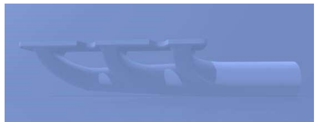
Fig 3 Exhaust Manifold STL File
