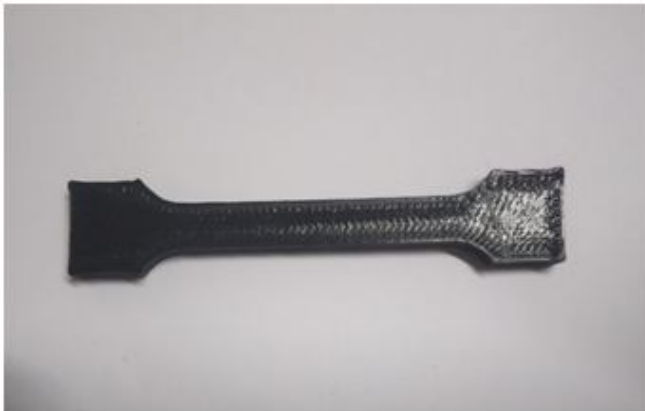
Fig 6 Printed tensile test specimen (Before testing)
