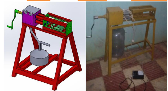
Fig. 1. Block diagram of design and fabrication for extracting cow dung pellets by extrusion method
