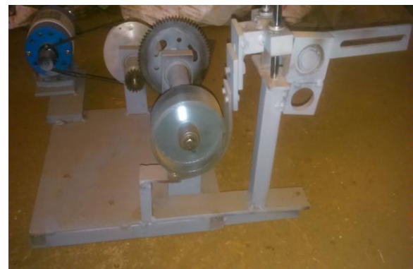
Fig.2 Test-Rig Used For Testing of Band Brake
