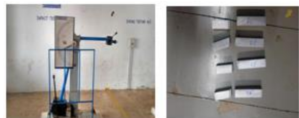
Fig 34: Izod impact testing machine and Broken specimens
