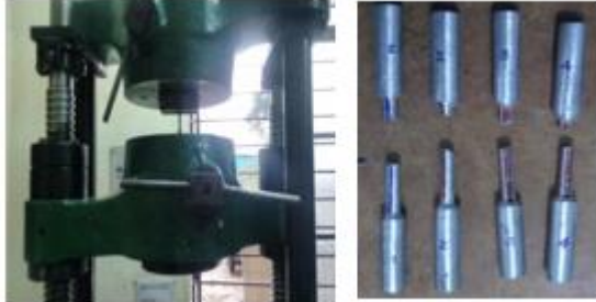
Fig 26 : Tensile specimen in Universal testing machine and Broken specimens
