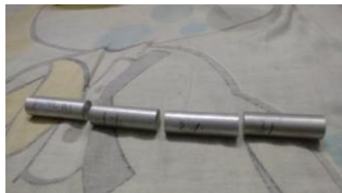
Fig 17: specimens for compression test
