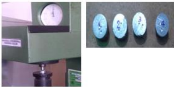
Fig 37: Brinell hardness test machine and specimens
