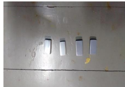
Fig 24: Polished specimens for microscopic study
