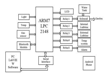
The overall block diagram of the proposed system is shown in figure.
