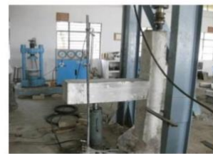
Fig 4.10 Beam Column Joint Test Set Up
