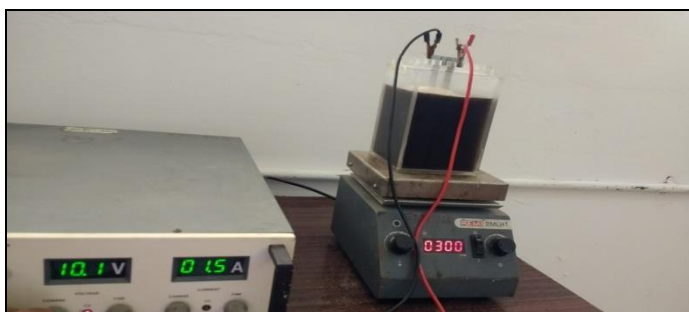
Plate 1: Experimental setup of Electro chemical coagulation treatment for distillery spent wash
