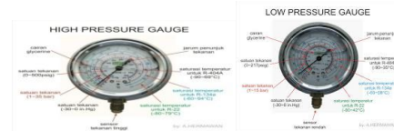
Fig.a) High pressure gauge (b) Low pressure gauge
