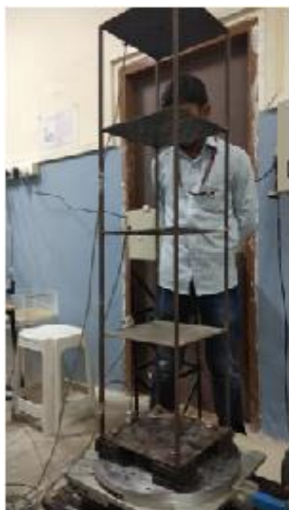
Figure 11: Experimental setup on a shake table for Base Isolated Structure
