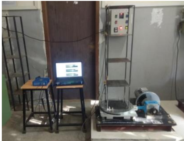
Figure 10: Experimental setup on a shake table for fixed base
