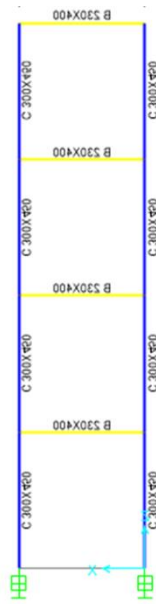
Figure 4: Elevation of the building with LRB
