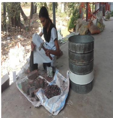
Figure 2: Crushing the over burnt bricks
