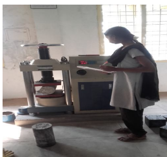
Figure 5: Compression testing machine-Cylinder testing
