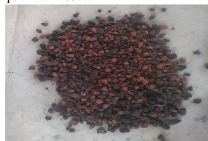
Figure 1: over burnt bricks
