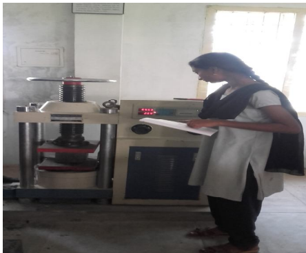
Figure 5: Compression testing machine-Cube testing
