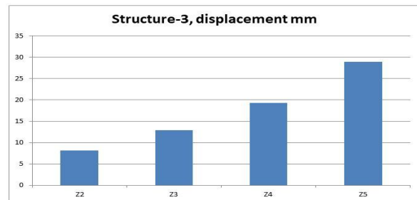
Chart 4.4: displacements in structure-3 in different zone
