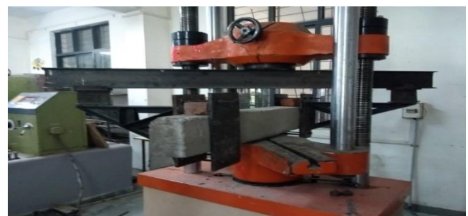
Fig.4 Test set up for rectangular spiral reinforcement beam Failure Pattern
