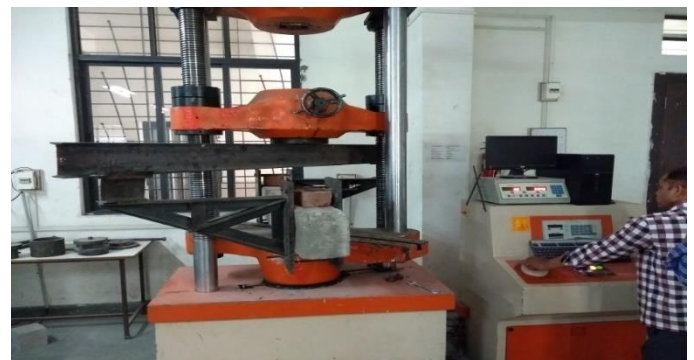
Fig.3 Test set up for control beam.
