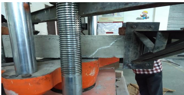
Fig.6 Crack pattern of rectangular spiral shear reinforced beam
