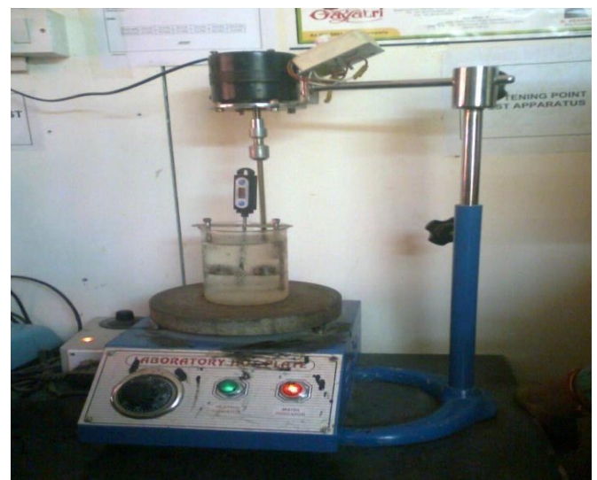
Fig 2 Softening test by ring and ball test
