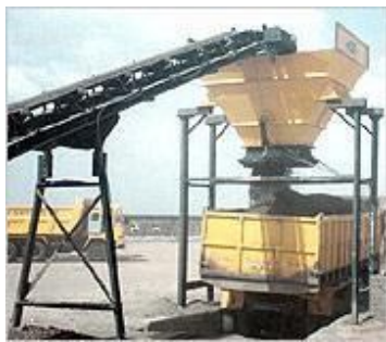
Fig 14 Surge Hopper/ Storage Hopper
