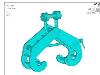
Fig 5.3: Boundary condition of displacement applied on end of crane hook.
