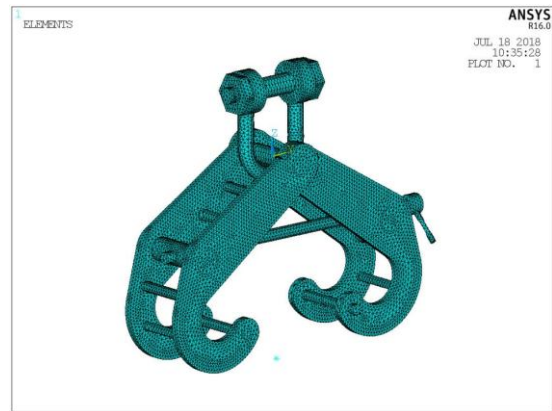
Fig 5.1: Meshed Ansys model of Total lifting clamp Assembly
