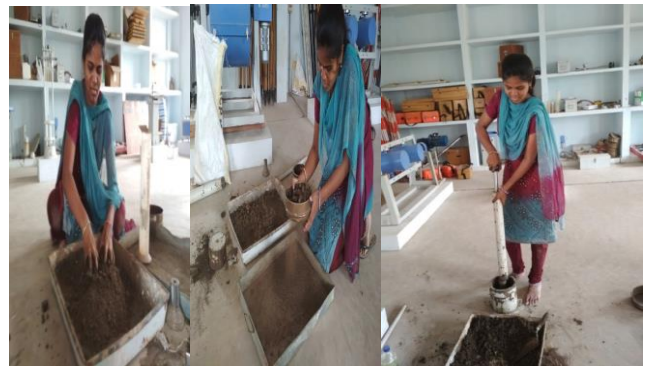
Plate 4.7 Author Conducting Modified Proctor Compaction Test
