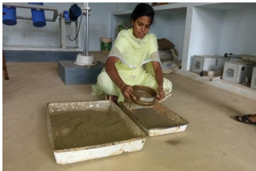
Plate 4.6 Author Conducting Differential Free Swell Test
