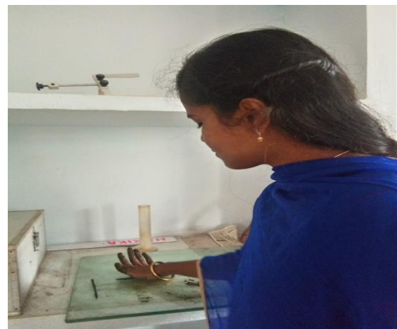
Plate 4.4 Author Conducting Plastic Limit Test
