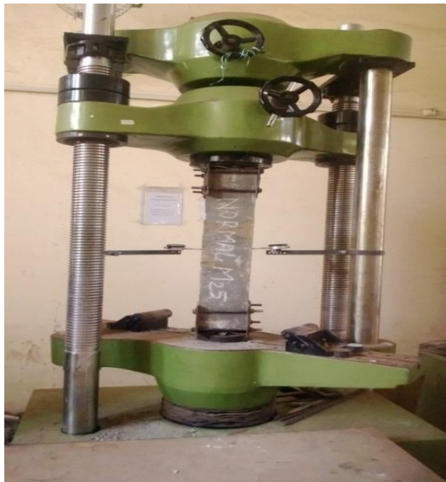
Fig 5.Hinge at top of column
