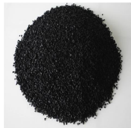
Fig.1 crumb rubber particle (size passing through 1.18 mm IS sieve and retaining on 600 \mu )
