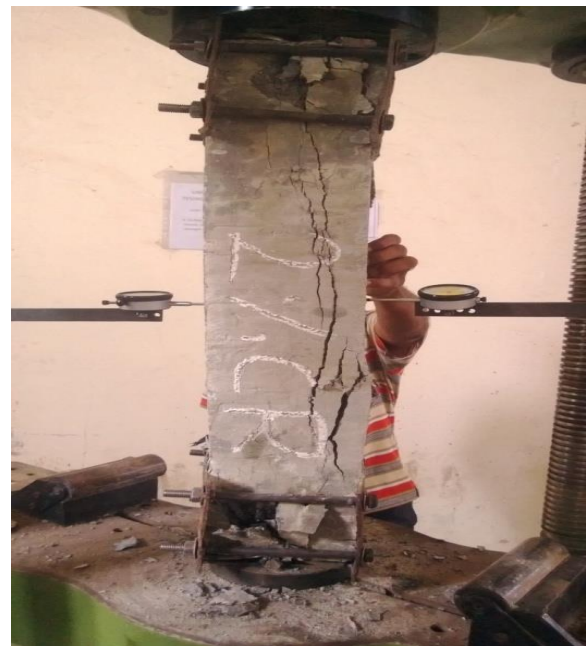
Fig 8. Failure of column specimen.
