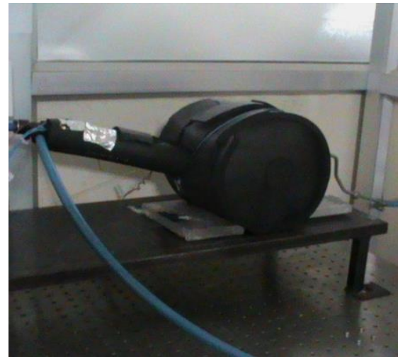
Figure 3: Evaporator covered with superlon insulation
