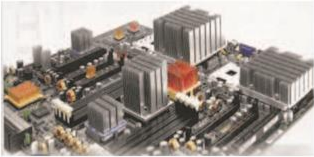
Figure 1.2: Application of heat sinks in an electronic enclosure [5]
