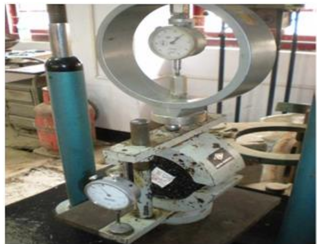
Figure5.1 Marshall Stability Test in Progress
