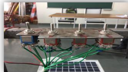
Fig- 3: Dedicated Toggle switch
