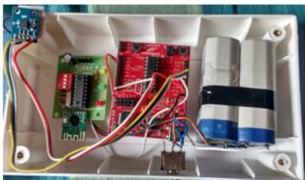
Fig.7: MSP development board interfacing with ADXL & RF Module
