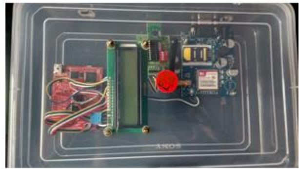
Fig.8: MSP development board interfacing with RF Module and GSM Module
