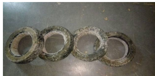
Figure 11. Concrete filled Tyre specimens
