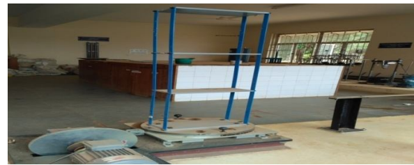
Figure 6. Shake table testing machine
