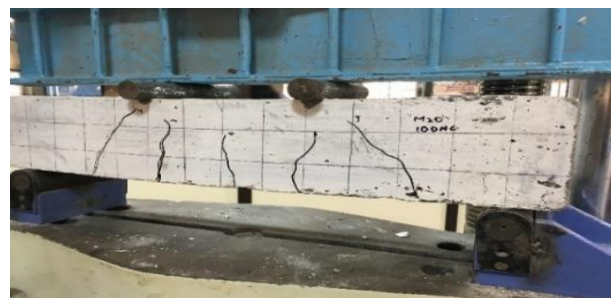
RCC beam specimen testing
