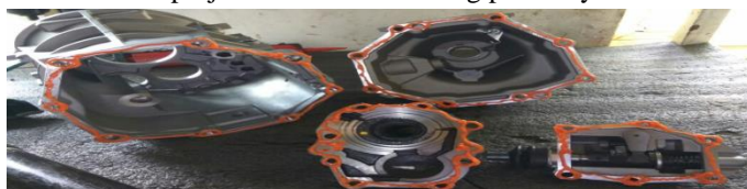
Figure 1. Uneven application of sealant by labor on casing
