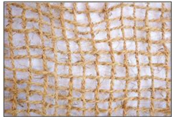
Fig 4.2 Grade I H2M6 Coir Geo textile
