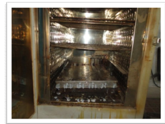
2.11 Excess resin mix Flowing out Of the Mould Fig 2.12 Placing the Mould In The Oven
