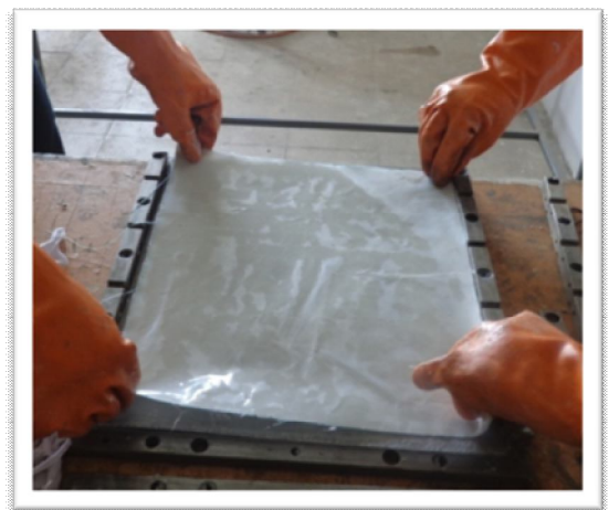
Fig 2.7 Consolidating Surface Mat Fig 2.8 Placing the First Ply
