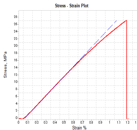
Flexural stress Vs Flexural Strain of 0.1wt % MWCNTs
