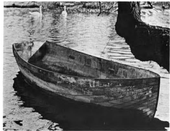
Fig1.2: Built in 1887, this Dutch Ferrocement boat was still afloat, in 1967, at the Amsterdam Zoo. (Cement, Amsterdam, The Netherlands)
