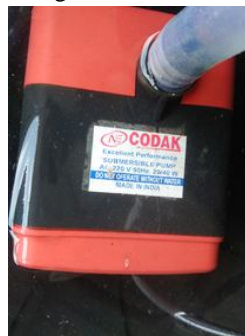
Figure:- Submersible Pump
