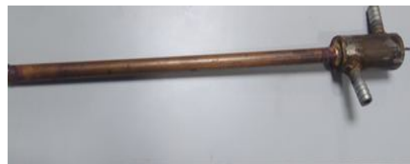
Figure:- Heat Pipe
