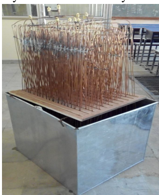
Figure: - Arrangement of CLPHPS with a dividing plate and Condenser Section duct.
