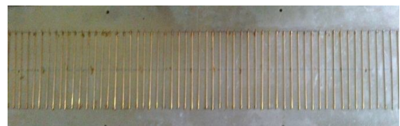
Figure 5.5 Photograph of transverse wires roughness geometry (p/e=10) on absorber plate
