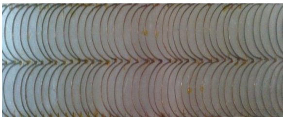
Figure5.9 Photograph of double arc wire roughness geometry (p/e=10) on absorber plate.
