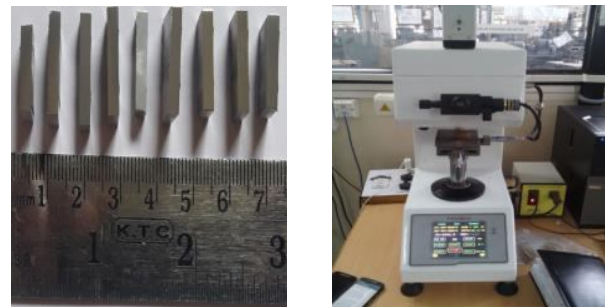
Fig 5. Microhardness Weld Specimen & Vickers Hardness Tester
