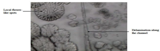
Flower-like spots in a UV-ozone treated chip after heat treatment
