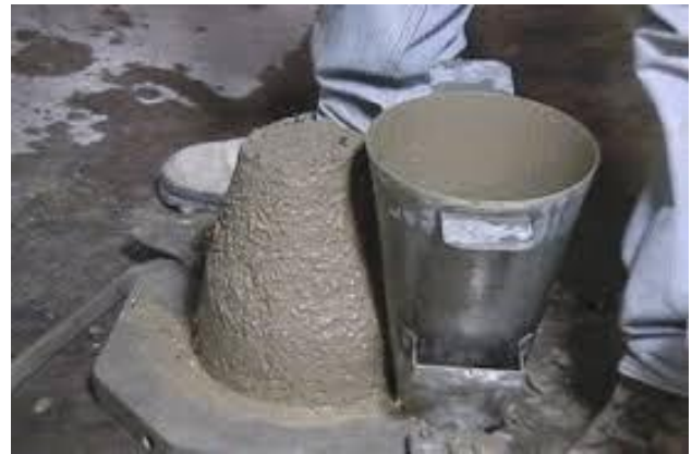
Fig 5 slump cone test
