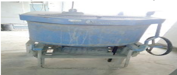
Fig: 4 Concrete Pan mixer used for mixing
