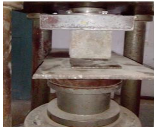
Fig 6 Compressive strength test setup
