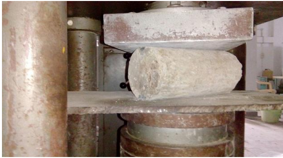
Fig 7 Split tensile strength test setup
