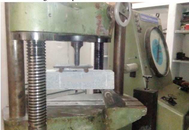
Fig 8 flexural strength test setup
