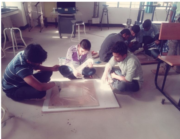
Figure 7: Fabricating By Hand Lay Up Technique
