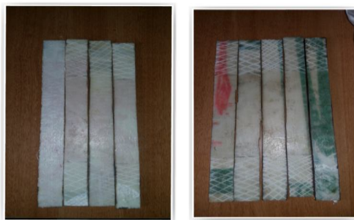
Figure 9: Specimen Tensile Tested for Set 1 and Set 2
