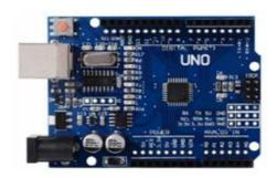
It belongs to ATmega 328 family. It composed of 14 functional pins, in which 6 are utilized for PWM outputs and remaining 6 for analog inputs one for the transmission and one pin for receiving the signals. A 5V supply is required to energise the controller board. The panel accepts the Arduino IDE software program which will be accepted by the controller present on board.
