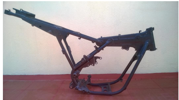
Fig.1: Bajaj Discover 135cc Chassis Frame
