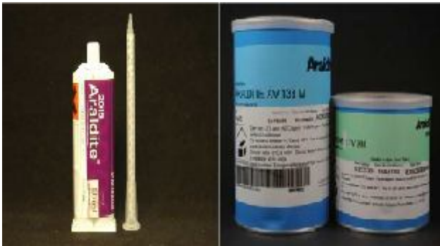
Fig.2: Araldite 2015 with the tube for application of the adhesive & Araldite AV138 with Hardener HV998
