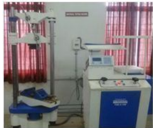
Fig.16: Experimental set up on Universal Testing Machine
