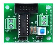
A L293D is used to control the two small dc motors in bidirectional way. This L293D motor driver will be controlled by the microcontroller.
