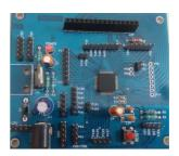
The controller used in this car washing is 64-pins, 11-ports R5F100LE microcontroller which is lead (Pb) free controller. Which Supports both flash memory programmingand on-chip debugging
