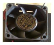
A fan is an electromechanical device. Mainly it is used for cooling/drying purpose. In this automatic car washing process it is used in drying section so that car will be dried and finally car will be available for delivery.
