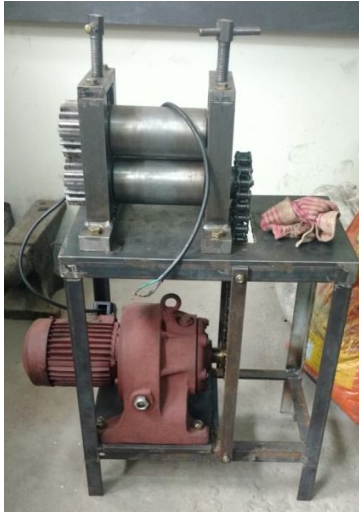
Figure.9 Developed Rolling machine
