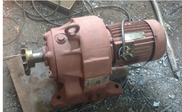
Figure.4 motor with reduction gear
