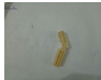
Figure 3.3: Glass FRP after charpy test
