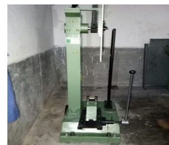
Figure 3.1: Charpy test machine used for specimen testing
