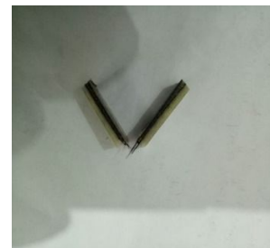
Figure 3.2: Carbon FRP after charpy test
