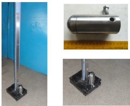
Figure 3.4: Drop weight test used for specimen testing
