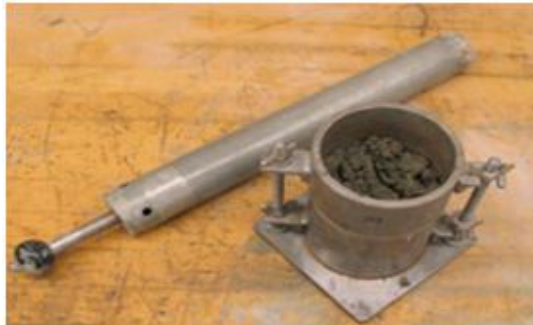
Plate 4.2 Conducting Modified Proctor Compaction test
