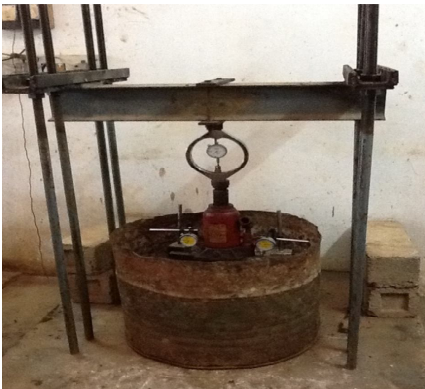
3.1.Prepared model tank for conducting Cyclic Plate Load test
