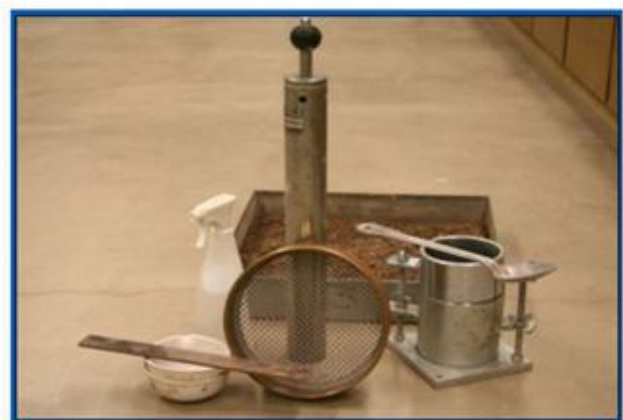
Plate 4.1 Preparing sample for modified Proctor Compaction test
