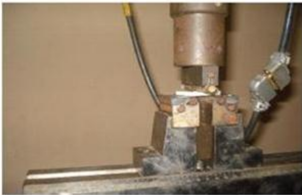
Fig2. Three point bend test setup and fixture.
