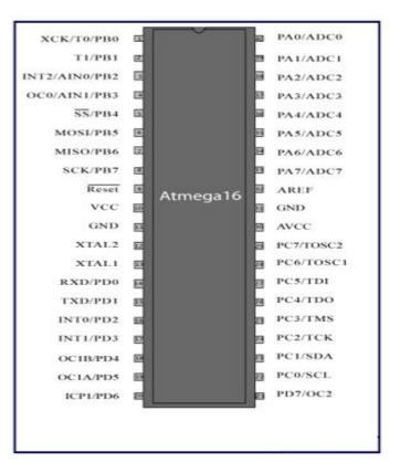
ATMEGA16 is a 8 bit microcontroller which is of Atmel's Mega AVR family with low power consumption. Atmega16 is based on enhanced RISC architecture with 131 powerful instructions. Most of the instructions execute in one machine cycle.
