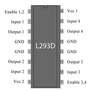
To drive the DC motors used for cutter as well as for moving the base frame of the agriculture robot there is a requirement of motor driver therefore L293D IC is used. This is a dual H-bridge integrated circuit(IC). This is used as a current amplification to drive the DC motors. This is a 16 bit IC used in both the directions. By using this L293D IC we can control from this IC maximum two motors from one IC.
