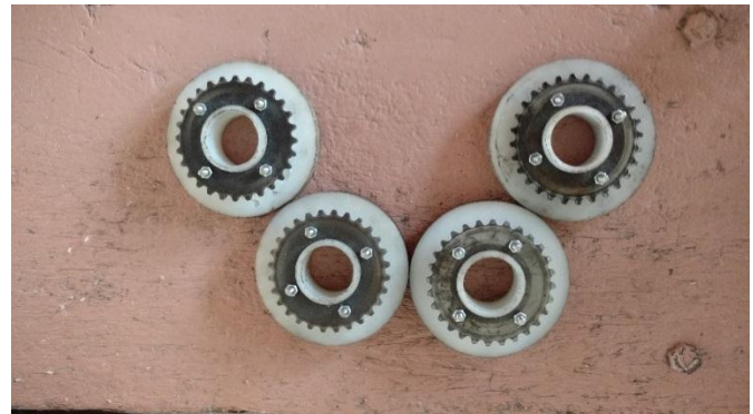
Fig. No.6Nylon wheel with Chain Sprocket
