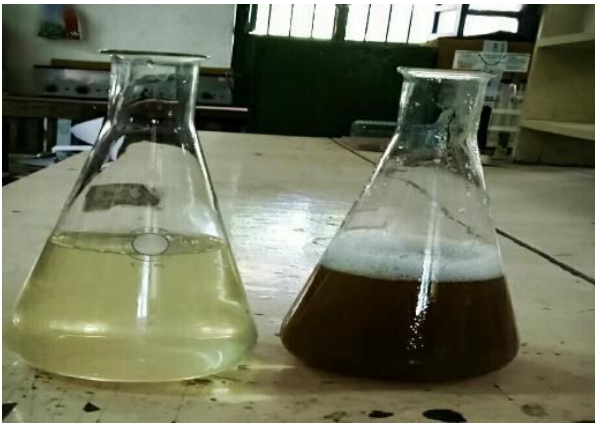
A Comparison of before and after treatment of Pulp and Paper Industrial Wastewater using MEMBR
