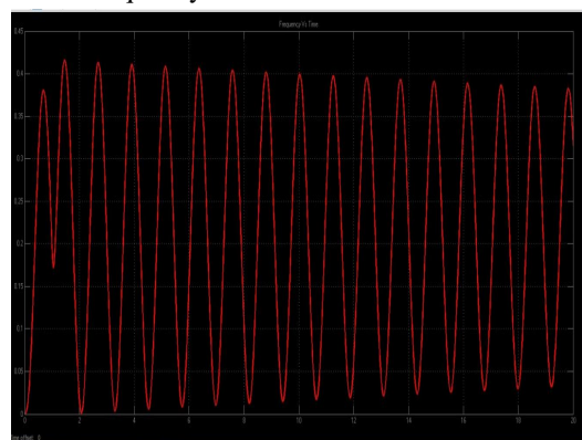
Figure 3 Response for open loop single area for change in frequency
