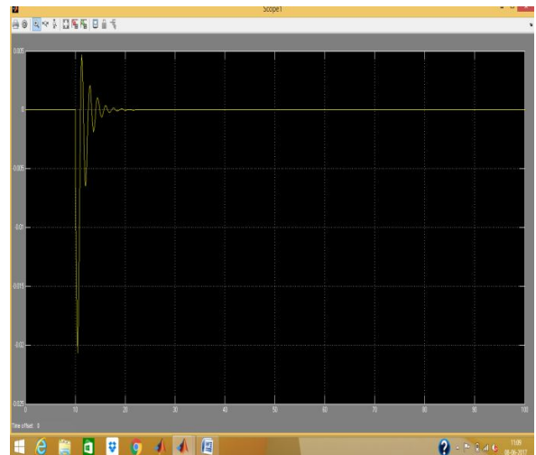
Fig 29 performance graph of change in frequency in area 2 using FLC
