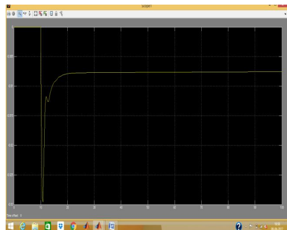
Fig 12 Response for Area 2 AGC system for change in Frequency
