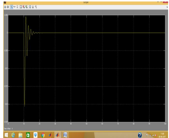
Fig 28 performance graph of change in frequency in area 1 using Fuzzy Logic controller
