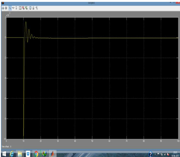
Fig 20 Response for Area 1 AGC system for change in Power
