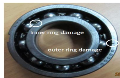
Figure 1: Inner and Outer ring faults of bearing
