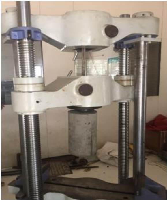
Figure 3: Pull Out test on cylinders
