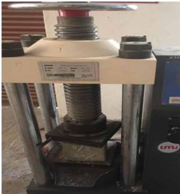
Figure 1: Compressive test on cubes
