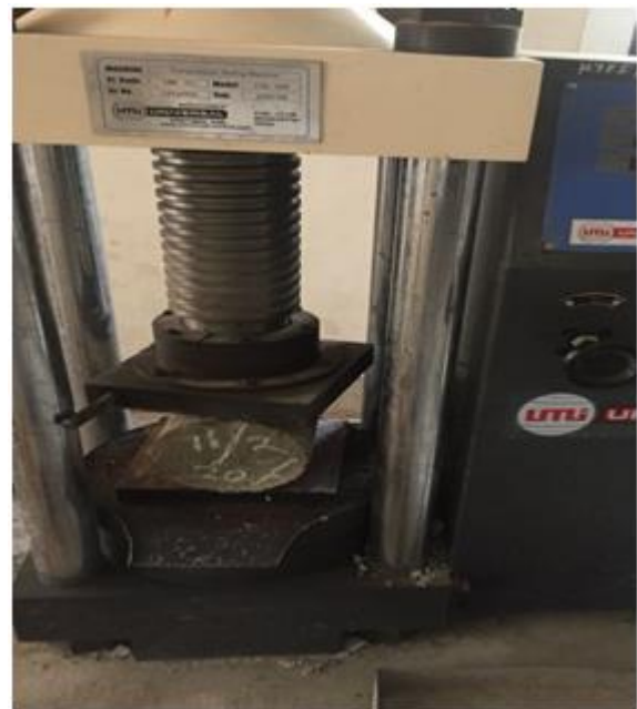
Figure 2: Tensile test on cylinders
