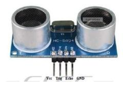
HCSR04 Ultrasonic sensor is utilized as a part of this undertaking as deterrent sensor or a range sensor. The extending separation of this module is from 2cm to 400cm. It as 4 pins: Vcc, Gnd, Trigger and Echo. Trigger is the yield flag created from the sensor, it goes every which way and when it hits or sense any protest or vehicle on their way, it considers it as a hindrance and sends a flag back to the controller and this flag is called as Echo flag. It works at 5V DC.
