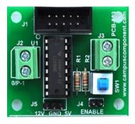
The L293D engine driver module is utilized to furnish an opportunity to interface with different applications. It works as Current enhancer, it acknowledges the low present and gives high yield current. This is acquired with a decent quality Printed Circuit Board (PCB).
