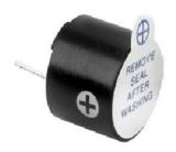
Signal is utilized as a sign gadget. It creates a signal sound to alarm vehicle driver that some hindrance is going ahead the path to the vehicle and educates him to back off or stop the vehicle to maintain a strategic distance from the vehicle crash and human passing. Its made up of Noryl material with a fixed structure, and is Black in shading. ix. LED:
