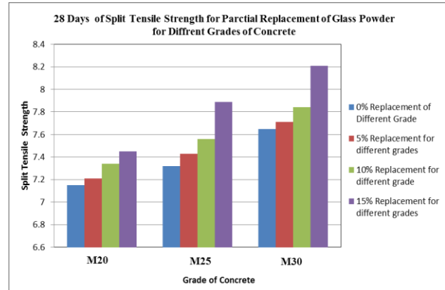
Fig 4.5: Bar Diagram for 28 Days Split Tensile strength for partial replacement of GP & FA for different Grades of Concrete.
