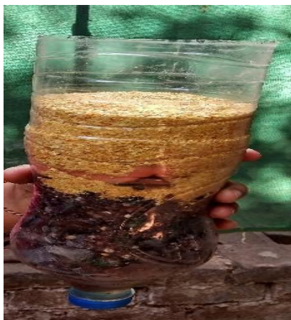
Figure No.1 Sand filter with low cost adsorbent
